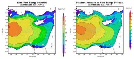
Figure 1. Mean values and deviation of wave energy potential in the Levantine Basin
