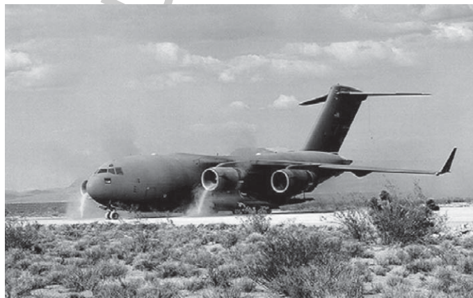
Fig. 7. Sand ingestion at high power settings.
