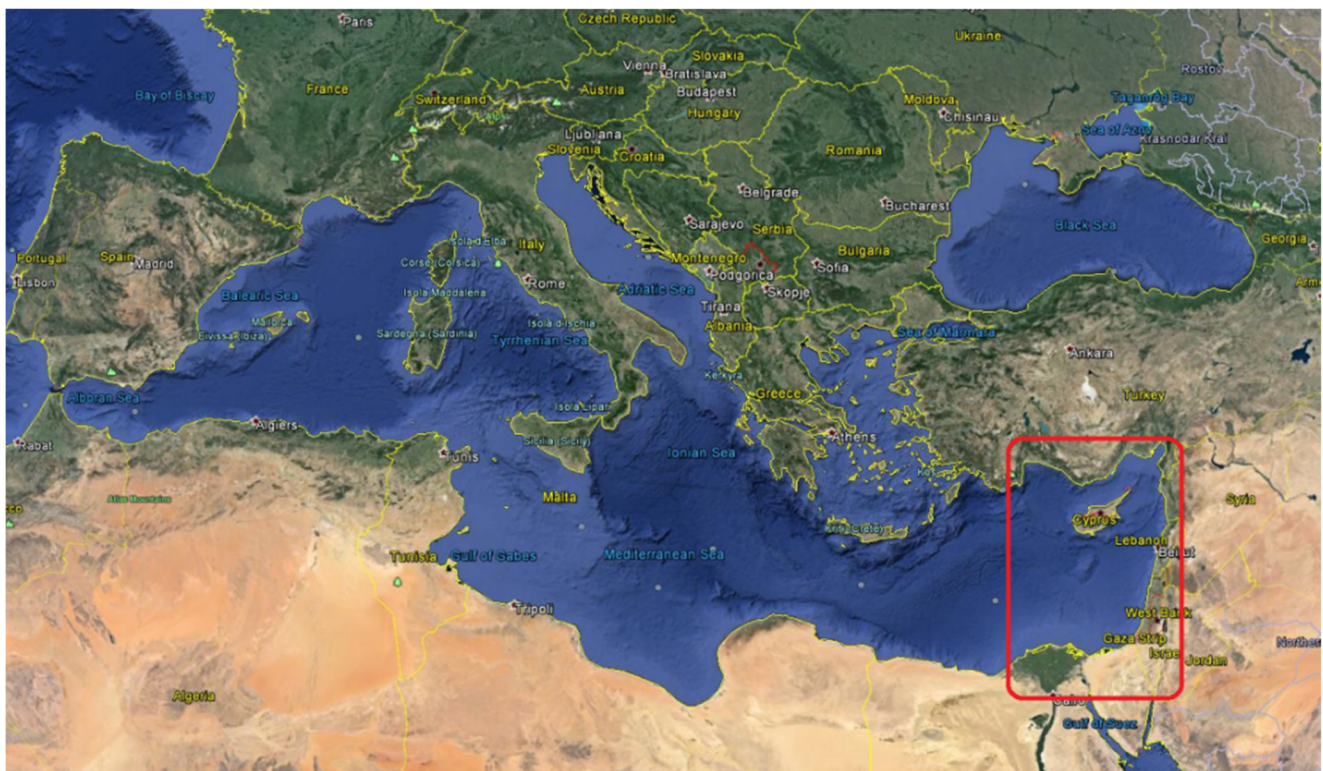
Fig. 2 The domains of the wave model: The coarser covers the Mediterranean and Black Seas while the second (denoted with the red rectangle) covers the high-resolution Levantine basin
