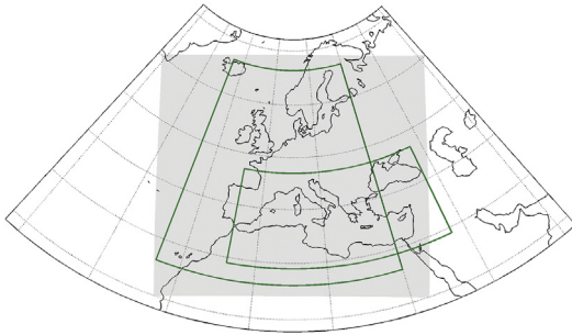
Fig. 1. The gray-shading indicates the SKIRON model domain. The green frames show the areas over which SKIRON passes wind data to the WAM model.
