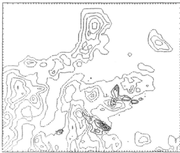
Figure 9 The mean annual concentrations ( \mu\text{g}/\text{m}^3 ) for total \text{SO}_2 , \text{NO}_x and TSP estimated for a gas-fired power plant at Keratsini.
