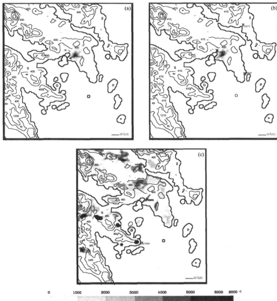
Fig 2. Hourly emission rates in 500 gr_moles/h intervals (a) anthropogenic VOC, (b) anthropogenic NO x and (c) isoprene, at 12.00 UTC of 7 July 1994.
